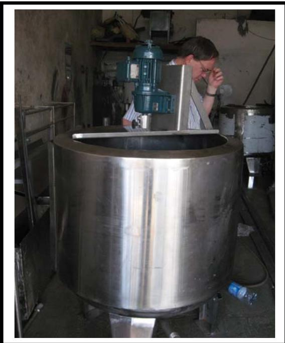
200lt Gaz powered Milk Heating vessel at Salhab Ice cream, Nabatieh, as part of the (LAISER) project.
