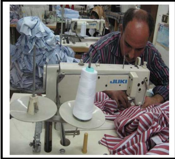
Direct Drive, High Speed, 1-Needle, Lockstitch Machine at Chic Top, Southern Suburbs of Beirut, as part of the (LAISER) project.
