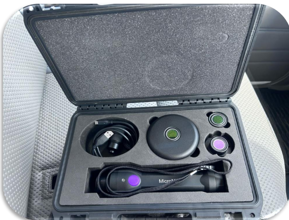
Zimbabwe: Micro Near Infra Red machine for falsified medicine surveillance © Dr Flora Zhou
