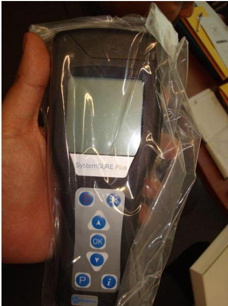
Luminometer for Biotrace
